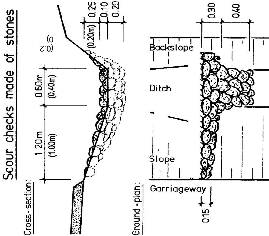
**FIGURE C.6 - MASONRY SCOUR CHECKS**
