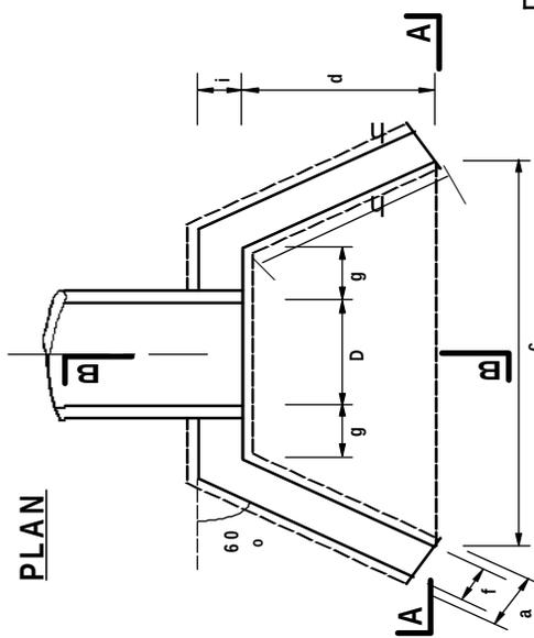
**FIGURE C.9 - HEADWALL TYPE 2 (DROP INLET)**
